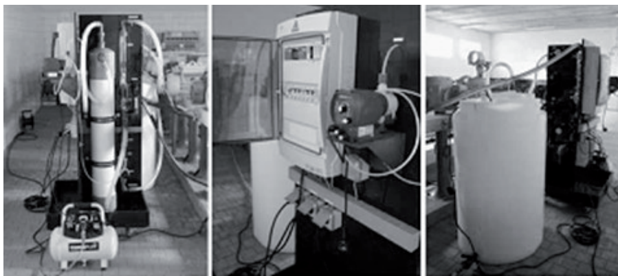
Fig. 4. A view of the ultrafiltration device, the membrane module itself, the control system, and the treated water storage tank.
